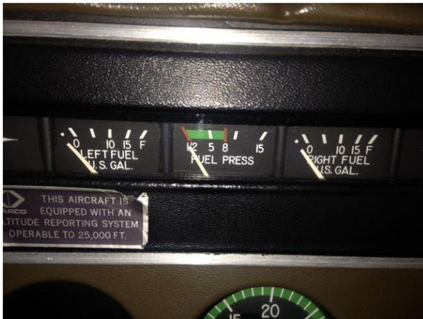
So, here’s the dilemma: If we assume Full is 25 (only 24 of which are useable) then why is the middle mark labeled “10”? Why is the  $\frac{3}{4}$  mark labeled “15”,  $\frac{3}{4}$  of 25 is 18.75 gallons, half of 25 is 12.5 gallons, not 10.  $\frac{3}{4}$  of 24 is 18 and  $\frac{1}{2}$  of 24 is 12. So, in any form the numbers are
